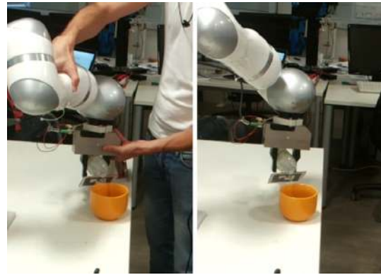
Fig. 4 Teaching and execution of the pouring action (NOA). In the teaching phase (left) the user drives the robot near the cup and pours water, while in the execution phase (right) the robot reproduces the movement
