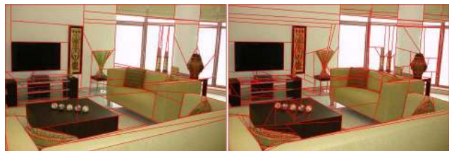
Figure 6. Partition complexity. We can produce partitions with varying numbers of polygons by tuning the sensitivity of the line-segment detector. Left partition with 113 polygons is sufficient for capturing the indoor structure and the main furnitures. Right partition (365 polygons) also captures smaller details as some patterns of the background painting.
