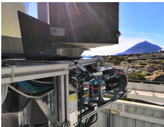
Figure 4. KISS instrument integrated on the QUIJOTE telescope in Tenerife. On the background the Teide volcano.
