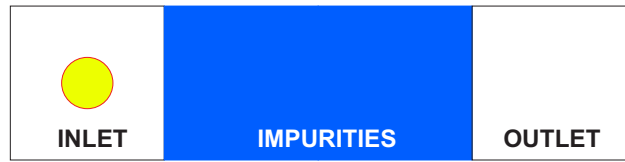
FIG. 4. Sketch of the domain setting used in our simulations of the propagation of a Gaussian wave packet through a porous medium.
