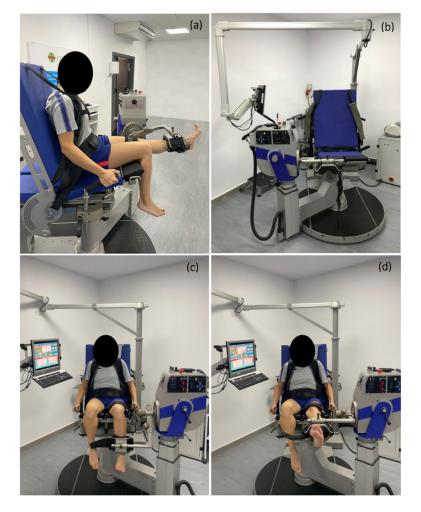
**Figure 1.** (**a**) Lateral view of the player with extension of the performing leg; (**b**) Frontal view of the Isokinetic dynamometer Isomed 2000; (**c**) Frontal view of the player with flexion of the performing leg; (**d**) Frontal view of the player with extension of the performing leg.
