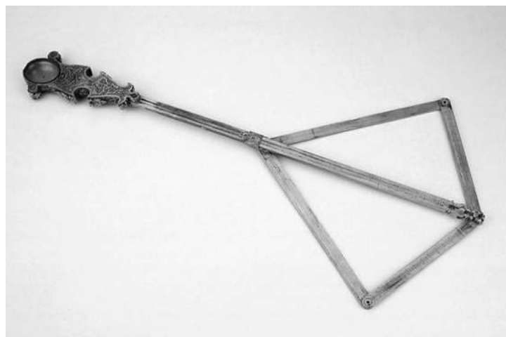
Figure 3. The radio latino, a multi-purpose instrument for warfare, by Giovanni Maria Mancini, c. 1600. Museum of the History of Science, inventory no. 37525.
