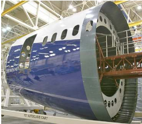
Figure 1-9 Boeing 787 fuselage barrel (Boeing)
