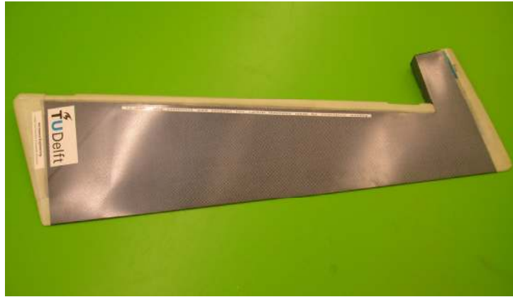
Figure 1-10 Euro-Enaer Eaglet General Aviation aircraft thermoplastic rudder
