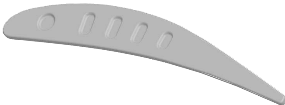
Figure 9-11 Model example showing the use of a nose or leading edge
