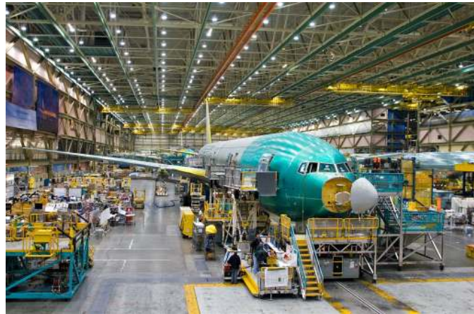
Figure 1-7 The Boeing 777 moving assembly line (Boeing)
