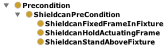
Figure 12: There are three preconditions to the ShieldCanInsertion skill. The skill has two feature frames (relative coordinate frames) as input parameters, where one is a reference object frame and the other is attached to the object in the gripper, i.e., an actuating frame. The first precondition is that the object with the reference frame has to be on the fixture. Secondly, the object with the actuating frame should be attached to the gripper, see Fig. 13, and finally, the position of the actuating object should be above the fixture. Imprecise geometrical relations such as “Above” are given concrete values by the Engineering System.
