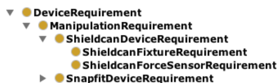
Figure 11: The device requirements of the skill ShieldCanInsertion are modelled in an ontology. The ManipulationRequirement which several skills inherit from, is that a gripper has to be mounted on the robot. The ShieldcanFixtureRequirement and the ShieldcanForceSensorRequirement list that there must exist a fixture and a force sensor that have to be vertically aligned (not shown in the picture).
