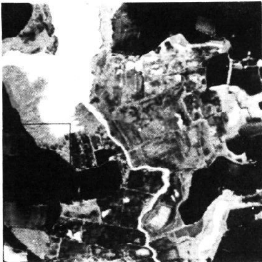
Figure 1 Aircraft Image Data of Barton Broads, Spring 1986. The figure shows a first principal component, 256 x 256 pixel image at 10m resolution.
