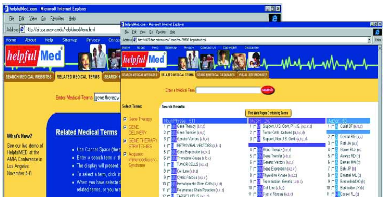
FIGURE 18 A 40 million term medical thesaurus was created using medical noun phrasing and co-occurrence analysis techniques. The system suggests medical terms relevant to users' queries, e.g., "Genetic Vectors" and "Gene Transfer" are suggested for "Gene Therapy." The system also maps user terms to relevant MeSH terms.
