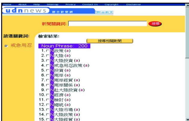
FIGURE 20 Related Chinese news topics are suggested based on statistical parsing and co-occurrence analysis techniques.
