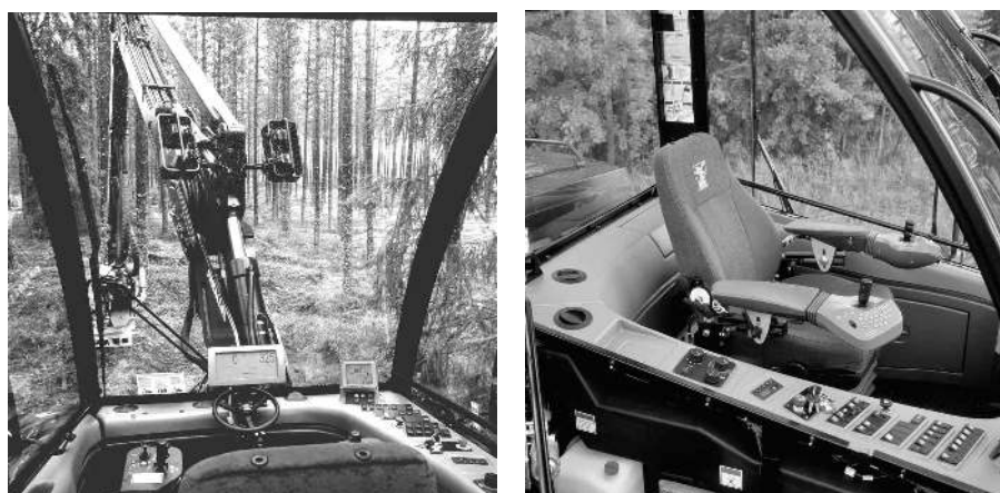
Figure 1. The revolution of work task requirements is well illustrated by the cockpit of a modern lumberjack with several computer and communication screens and control devices. Photos courtesy of Timberjack Group.
