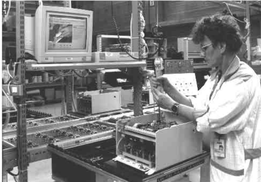
Figure 16. The support system was brought directly into assembly line work sites. The system was controlled by a bar code reader that the employees were more familiar with than the mouse. Picture courtesy of ABB Industry Ltd.
