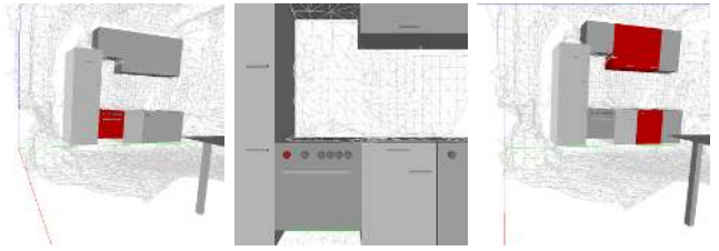
Fig. 5. Results of queries for objects that can be used for cooking food (left), for parts of the oven that cause a Boiling event (center) and for objects that contain drinking vessels (right), visualized by the graphical user interface of the knowledge processing system.
