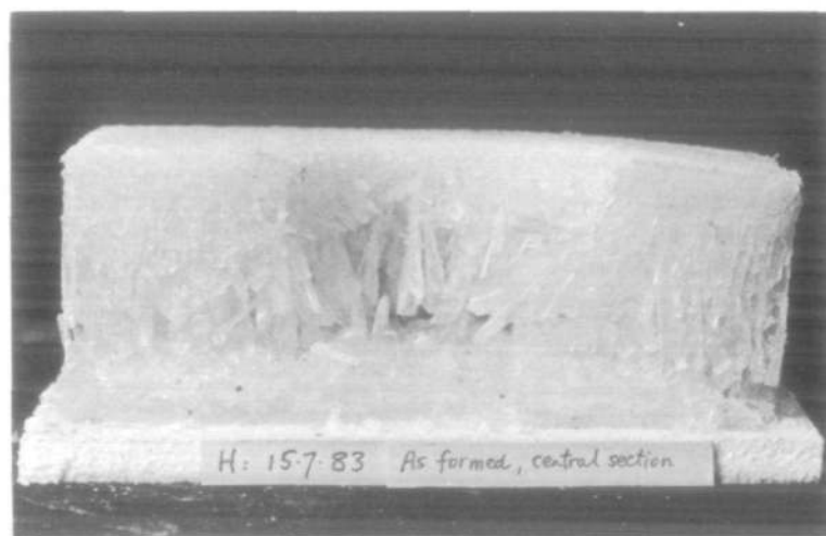
FIG. A6. The crystal block formed in run H, showing the hole left below an air bubble trapped at the roof. This hole later filled with solid eutectic, which was allowed to melt and run out before the photograph was taken.
