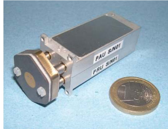
FIGURE 9: Tx/Rx active module connected to the radiating element.
