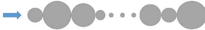
FIGURE 1. Schematic representation of a granular chain, with an impulsive force applied to the first element.
