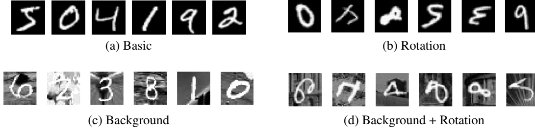
Figure 2. The MNIST dataset and its variations. (a) the basic MNIST dataset; (b) the digits were rotated by an angle generated uniformly between 0 and 2\pi . (c) a black and white image was used as the background for the digit image; (d) the background perturbation and the rotation perturbation are combined.
