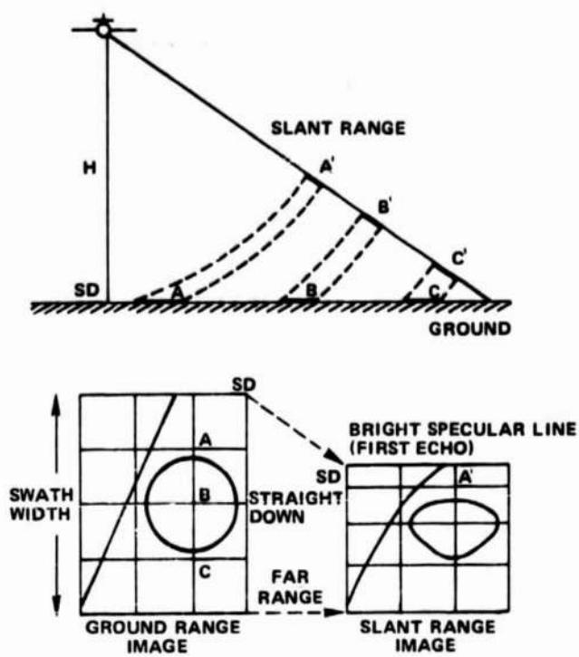
Figure 2. Slant Range Relationship for a SAR
