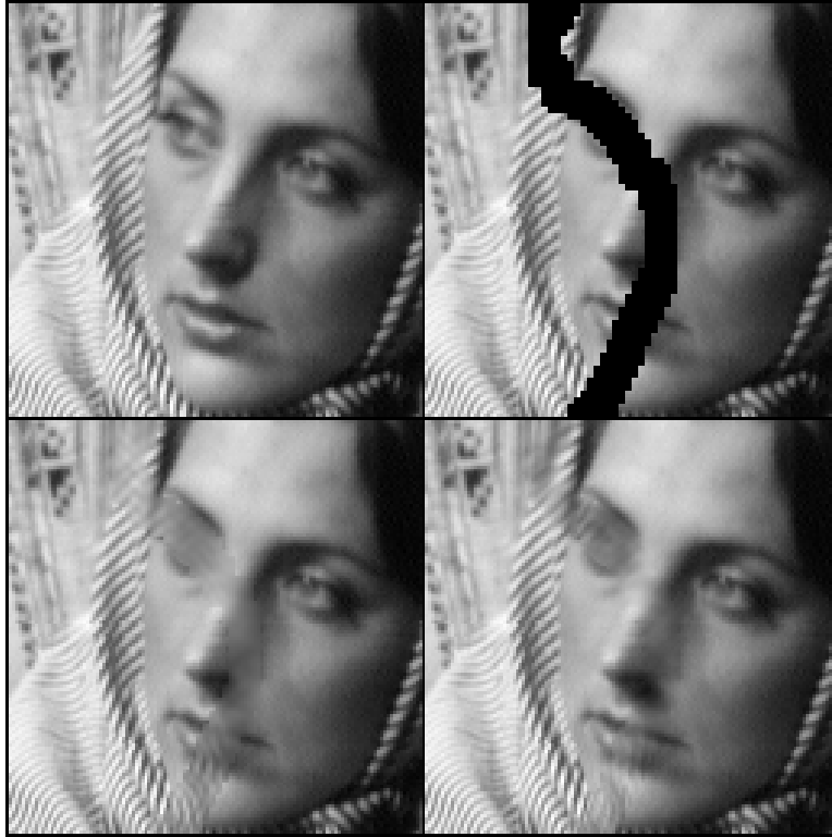
Figure 9. Application of \ell_0 -GM to in-painting. Top left , original Barbara image, cropped to 128 \times 128 starting at (301,50). Top right , degraded observation. Bottom left , result using dynamic soft-thresholding 11 (PSNR of the estimated pixels is 23.31 dB). Bottom right , our result (23.61 dB). Representation used is 6-scales Curvelets.
