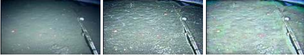
Figure 3. Multi-scale process inputs. Left: original OceanDark sample. Center: first input, an image enhanced using the contrast-guided CCI and A_{LCG\infty} with m = 5 . Right: second input, an image enhanced using the contrast-guided CCI and A_{LCG\infty} with m = 30 .
