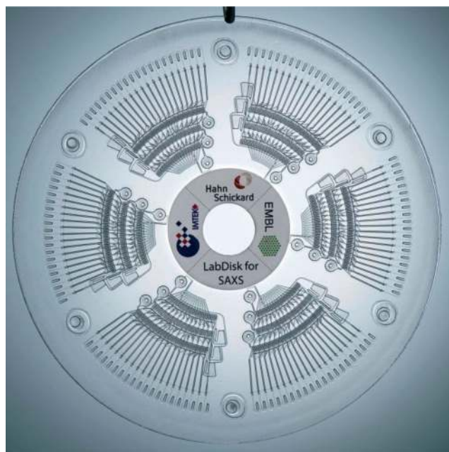
Fig. 1 LabDisk for SAXS. Each of the six segments includes the aliquoting of the three input liquids, the combination and the mixing in different predefined concentrations. The mixtures then reside in the read-out chambers. Read-out can be performed on disk in a synchrotron beamline. The fluidic function of the segments is explained in Fig. 2–5.
