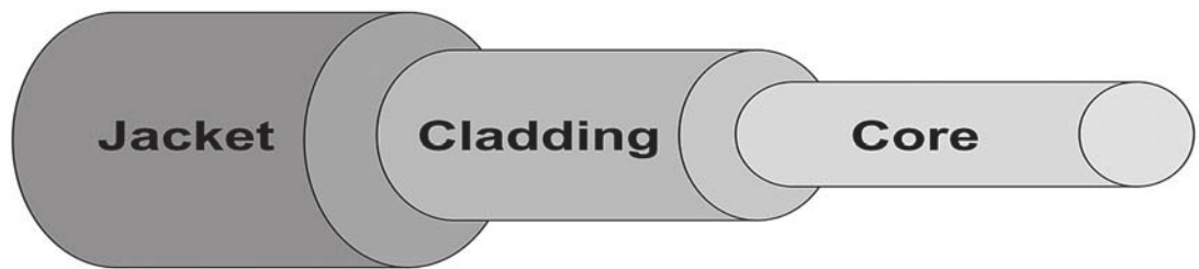
Figure 6: Basic structure of optical fiber.
