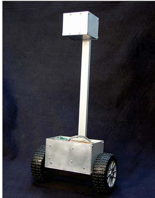
Figure 3. Mini-Segway process. This process was developed as a project in the real-time systems course in 2003 by four students. The project included mechanical design, construction, electrical circuit board fabrication, Atmel microprocessor programming, and control design.
