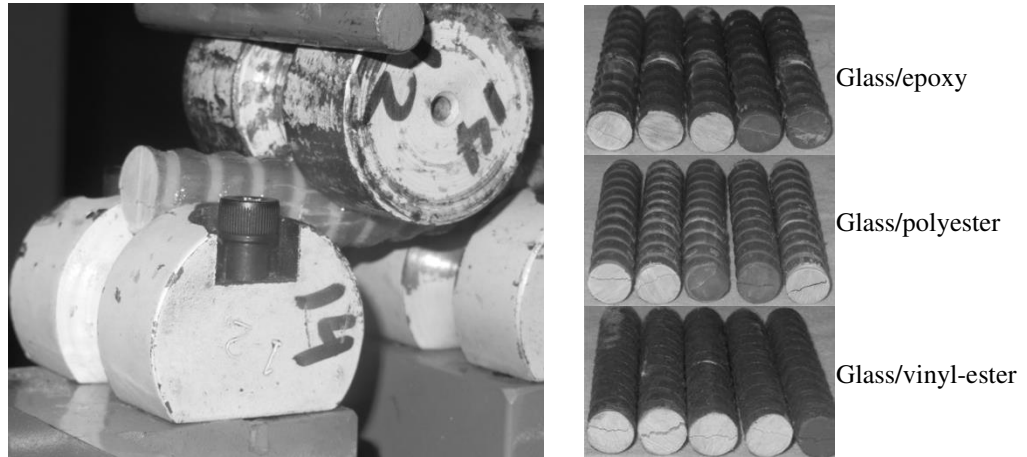
Figure 5. Setup for short-beam testing and typical failure mode: (a) test setup; (b) failure mode
