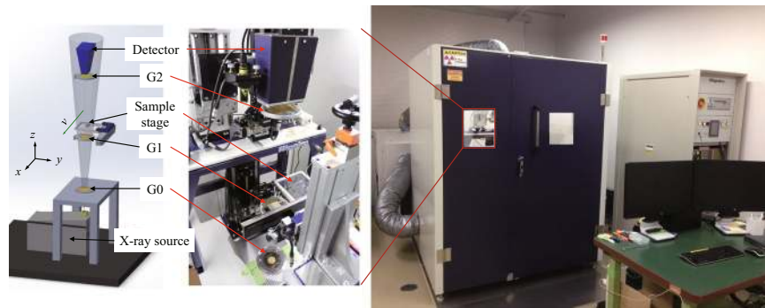
Figure 1. Schematic of the X-ray phase scanner prototype system (left) and its pictures (right).
