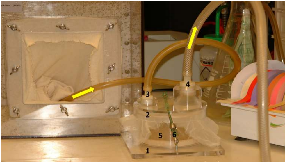
Figure 11. Vacuum-powered aspirator (Precision Plastics, Beltsville, MD, USA) for rapid transfer of large numbers of blood-fed flies from holding cages to ovipots: 1. Holding plate; 2. Aspirator lid with attached transfer and vacuum hoses; 3. Transfer port and transfer hose; 4. Vacuum port and vacuum hose; 5. A 500-ml ovipot nested in the depression of the holding plate; 6. Elastic securing cord hooked into screw eye ring on the holding plate. Arrows indicate the direction of air flow. (Photo by T. Rowland).
