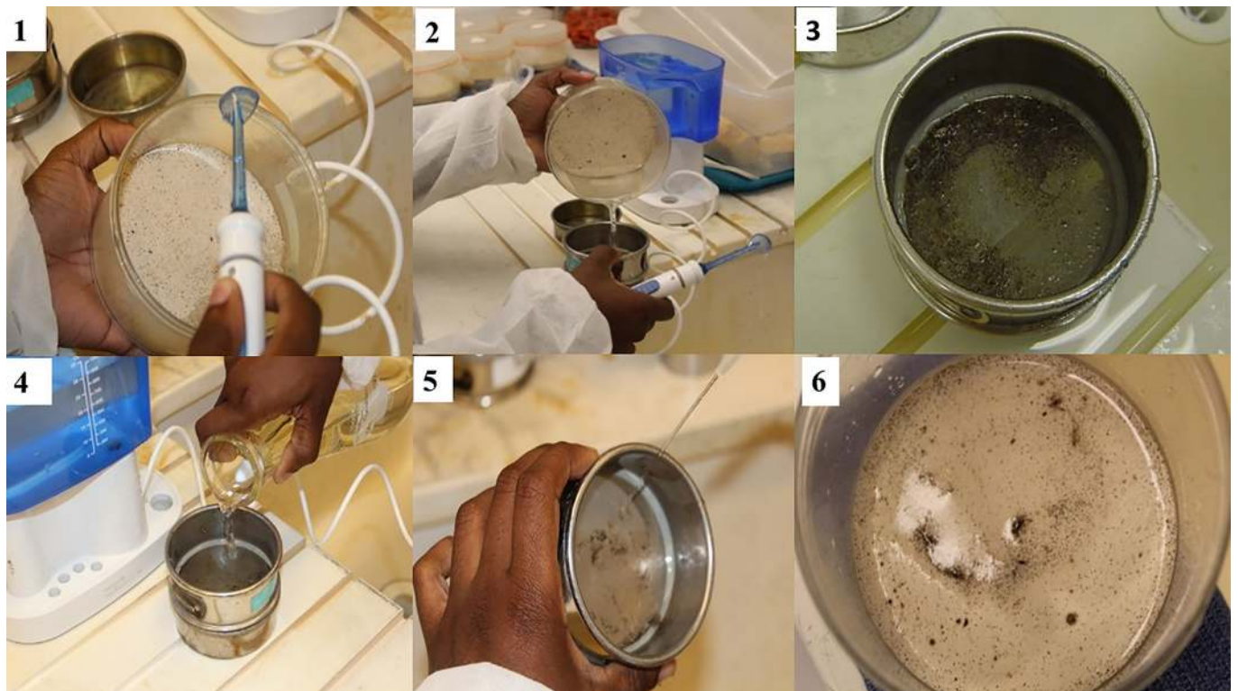
Figure D. 1 – Sand fly eggs are dislodged from the plaster surface in the bottom of an ovipot using a Waterpik ® (oral irrigator) with fan-spray attachment; 2 – The egg/water suspension is flushed into the appropriate colour-coded sieve; 3 – Eggs in a sieve that have been flushed from an ovipot; 4 – The sieve containing eggs is nested in a soaking pan filled with 1% sodium hypochlorite; 5 – After soaking, the eggs are flushed to one side of the sieve with a squirt bottle; 6 – The eggs are flushed from the sieve and distributed evenly over the plaster surface in the bottom of a clean ovipot. (Photos by T. Rowland).
