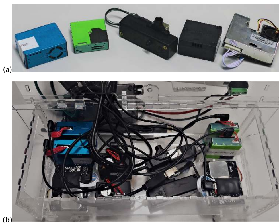
Figure 1. (a) Picture of the sensors tested from left to right: Plantower PMS5003, Sensirion SPS030, Alphasense OPC-R1, Honeywell HPM115S0 and Novafitness SDS018. (b) Position of the sensors tested within each air quality monitor. From left to right, top to bottom: two Plantower PMS5003, one Novafitness SDS018, two Honeywell HPM115S0, two Alphasense OPC-R1, two Sensirion SPS030 and one Novafitness SDS018. All the inlets are facing down.
