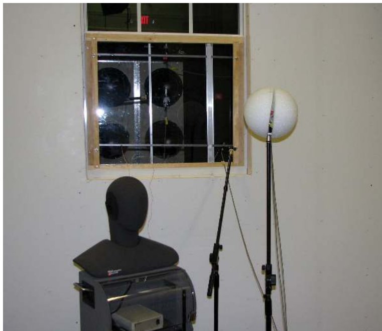
Figure 2. Recording of window rattles in the Gulfstream Acoustic Test Facility (ATF).
