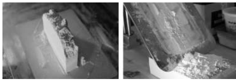
Figure 2: Left: Free standing column with view onto the top. Sides are straight, top is uneven; Right: flour pile ("rubble pile") after column collapse
