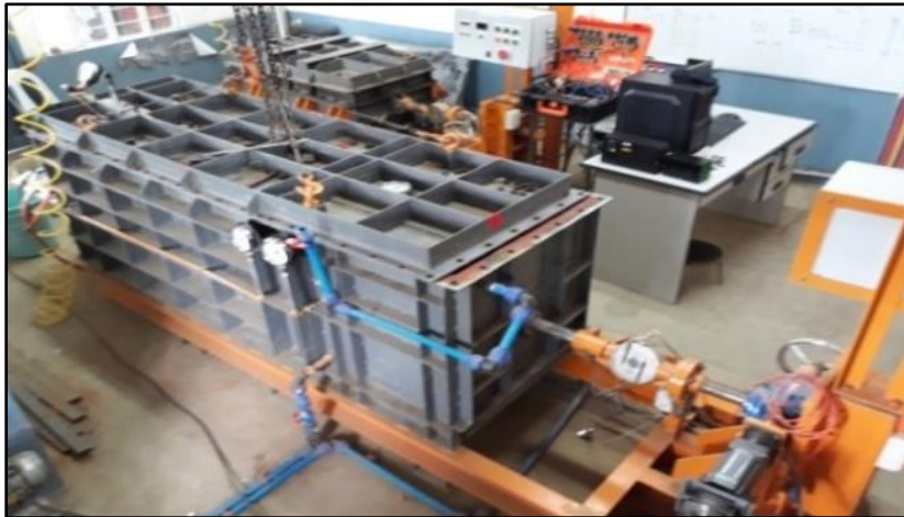
Figure 3. Fully automated large-scale pullout box with submerged capability
