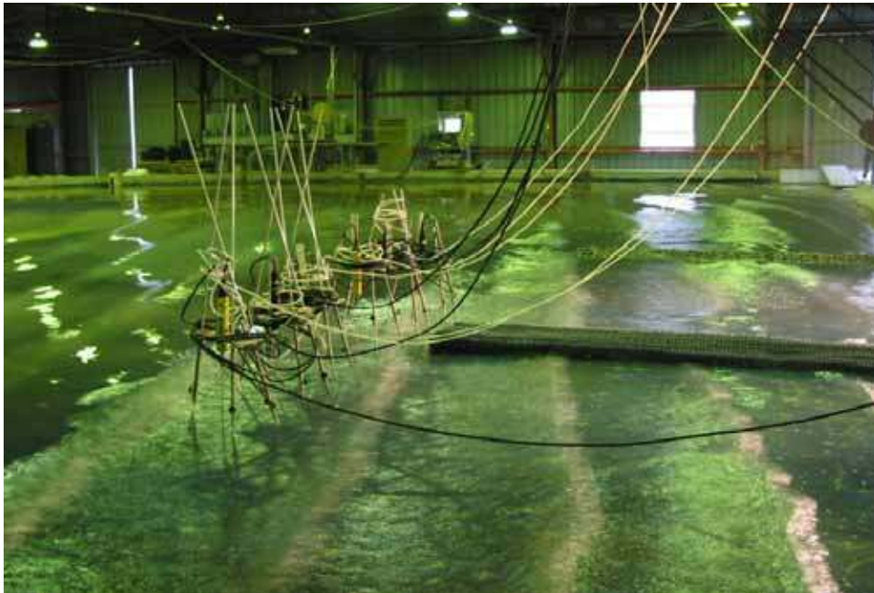
Figure 12. Current meters seaward of jetty
