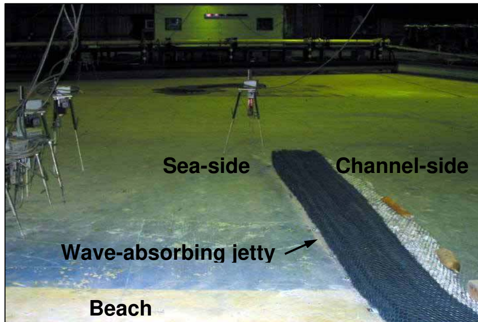
Figure 9. Wave-absorbing jetty perpendicular to shore in physical model
