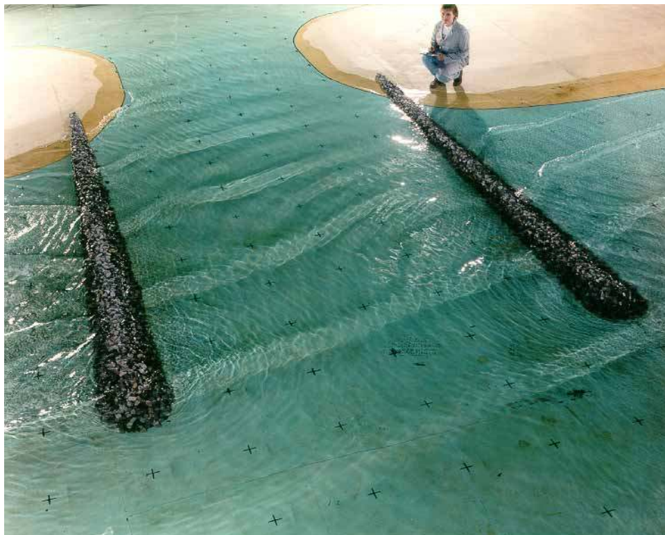
Figure 5. Idealized inlet entrance channel with oblique wave approaching inlet (spacing 0.62 m between "+" marking on research facility basin floor)
