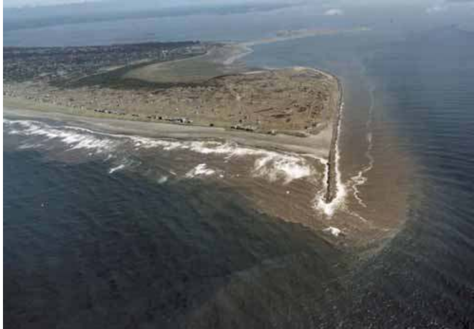
Figure 1. Wave-generated longshore currents entering Grays Harbor, WA, during flood tide
