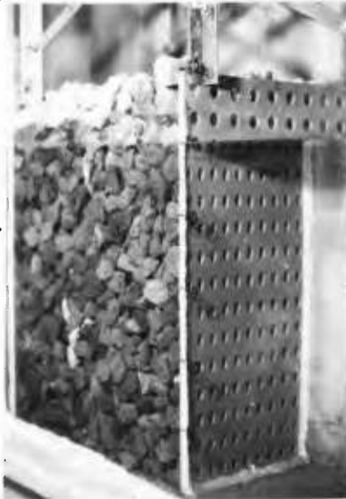
Photo. 2 Rubble Breakwater with Perforated plates
