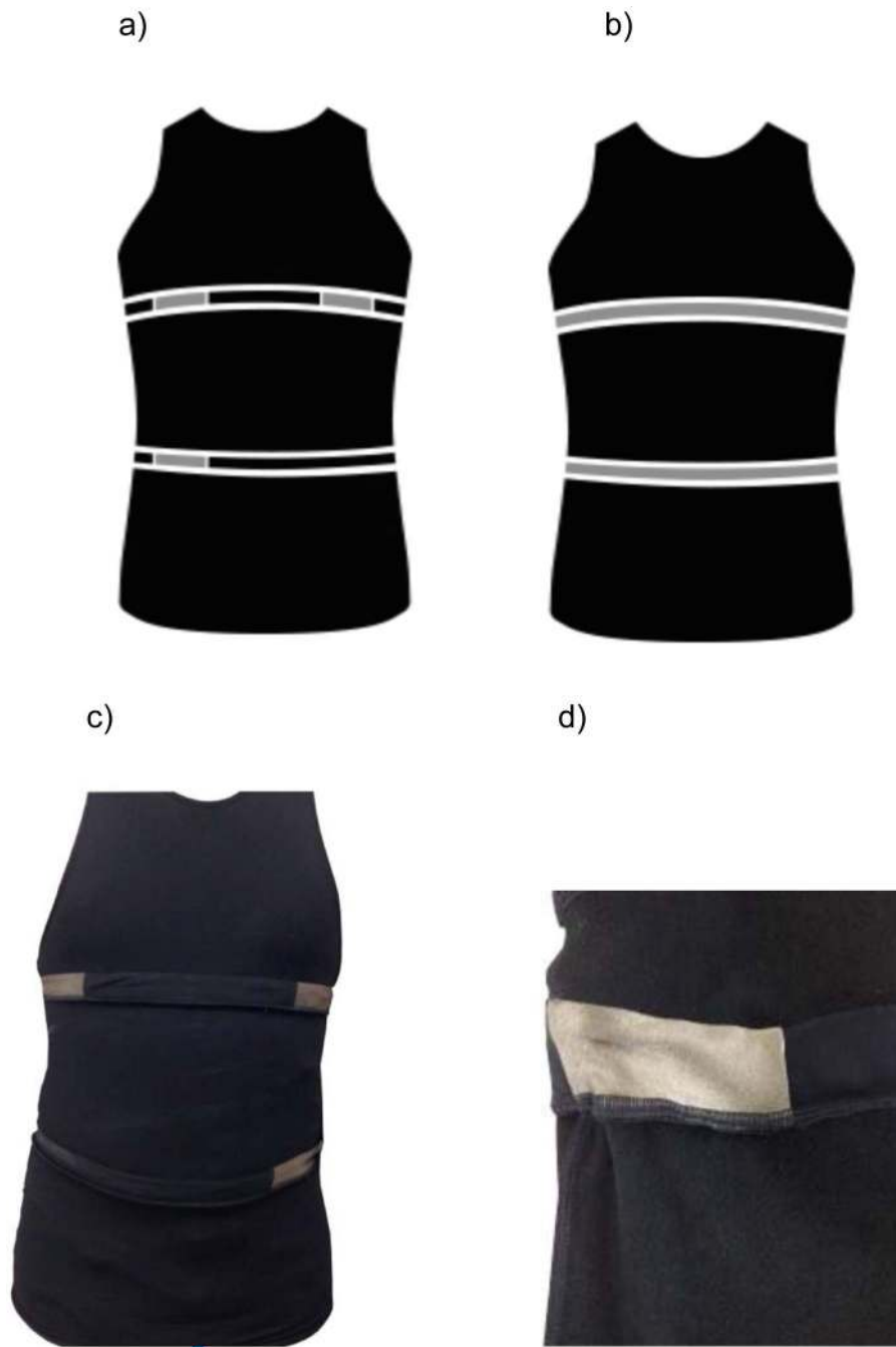
Figure 1. a) Cardiac sensors of the Hexoskin shirt; b) respiratory sensors of the Hexoskin shirt; c) Front inside view of the Hexoskin shirt; d) close up of the textile electrodes around the cardiac sensors.
