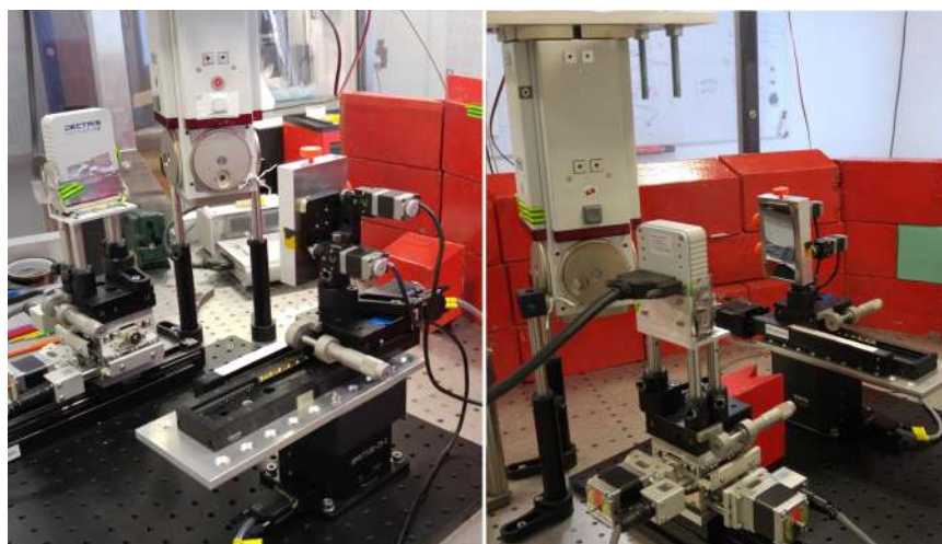
FIG. 2. An actual absorption measurement setup of the spectrometer without the shielding.
