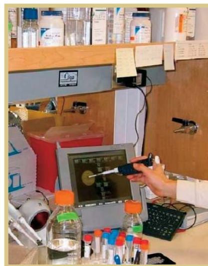
Figure 4. A minimally configured Labscape work area, including a touch-tablet computer, barcode scanner, numeric keypad, and small wireless keyboard.
