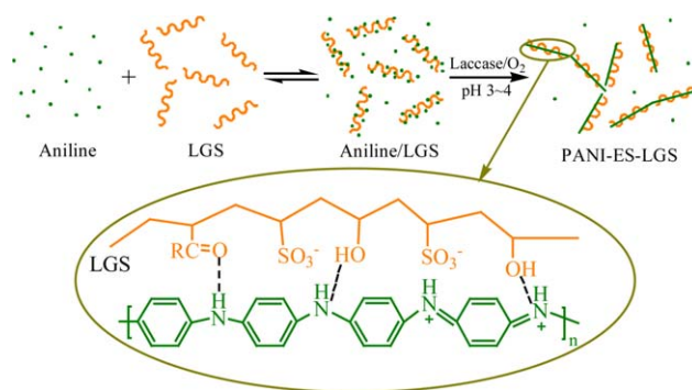
Figure 11. Schematic diagram of laccase catalyzed polymerization of aniline in LGS template system. [Color figure can be viewed in the online issue, which is available at wileyonlinelibrary.com .]
