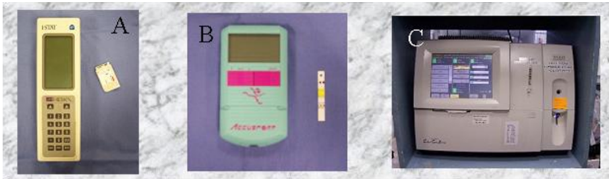
Figure 1: Three common point-of-care lactate analyzers in veterinary medicine. (a) i-Stat, (b) Accusport, (c) Nova chemistry analyzer.
