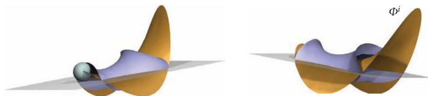
Fig. 13 The anticaustic map provides the transfer from an isotropic Willmore surface \Phi^i (graph z = f(x, y) of a biharmonic function f ) to a Lie-transformed Laguerre minimal surface \alpha(\Phi) (shown in purple). The latter surface is orthogonal to rays obtained by reflecting the z -parallel rays at \Phi^i . The surface \alpha(\Phi) is constructed as the envelope of spheres centered on \Phi^i and touching the xy plane. One such touching sphere is shown on the left.
