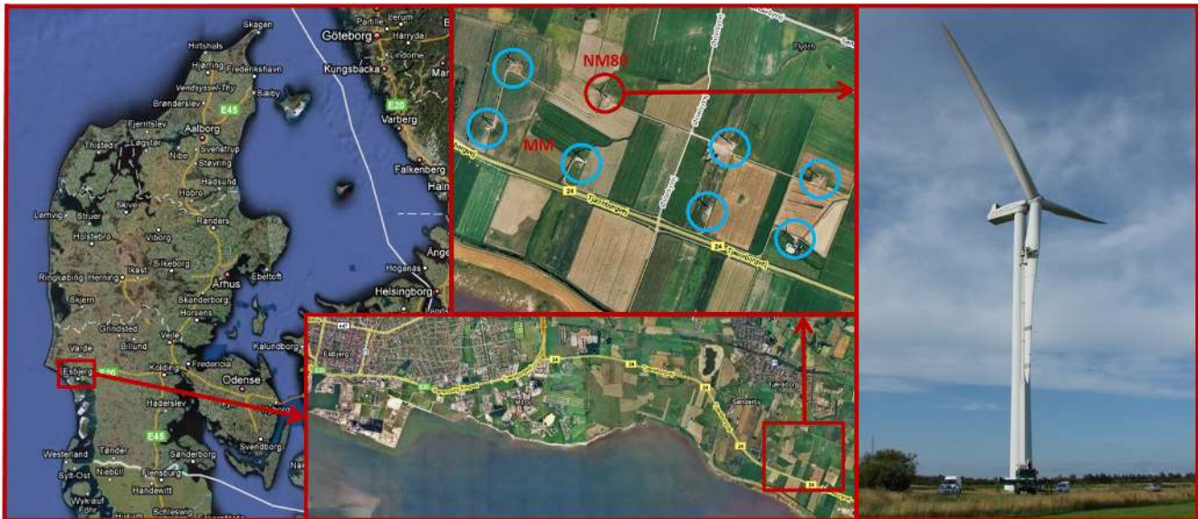
Figure 1. Map of the site approx. 10 km southeast of Esbjerg (© Google Maps 2007). The test turbine, NM80, is situated in a small wind farm at Tjæreborg along with seven other wind turbines of around 2 MW in size. The other turbines are circled with blue and the test turbine is marked by the red circle. The meteorology mast is shown by the “MM” denotation in the picture.
