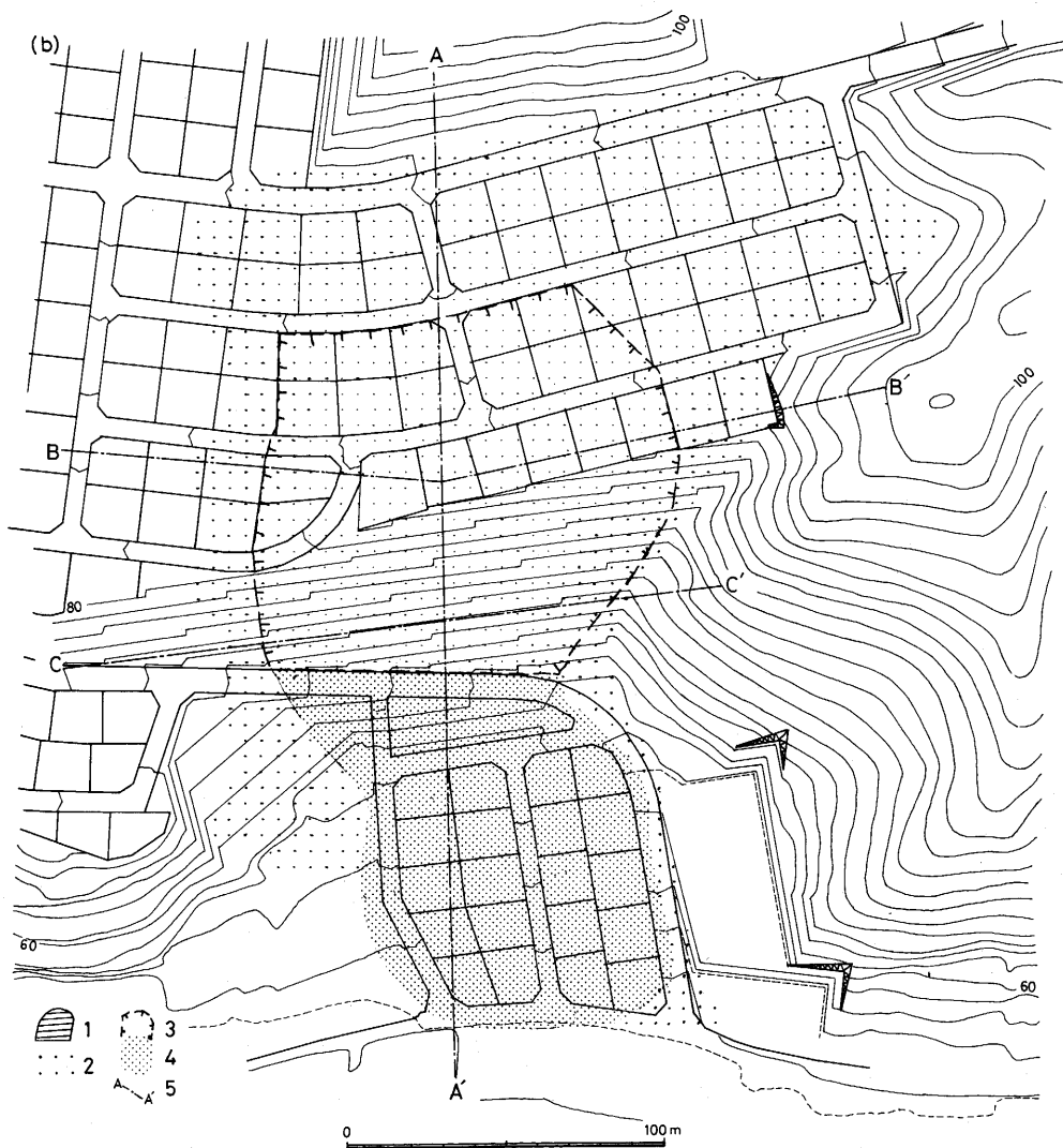
Fig. 14 Landform modification and earthquake-induced landslides in a residential area in Shiroishi, Northeastern Japan (Tamura et al., 1978).
