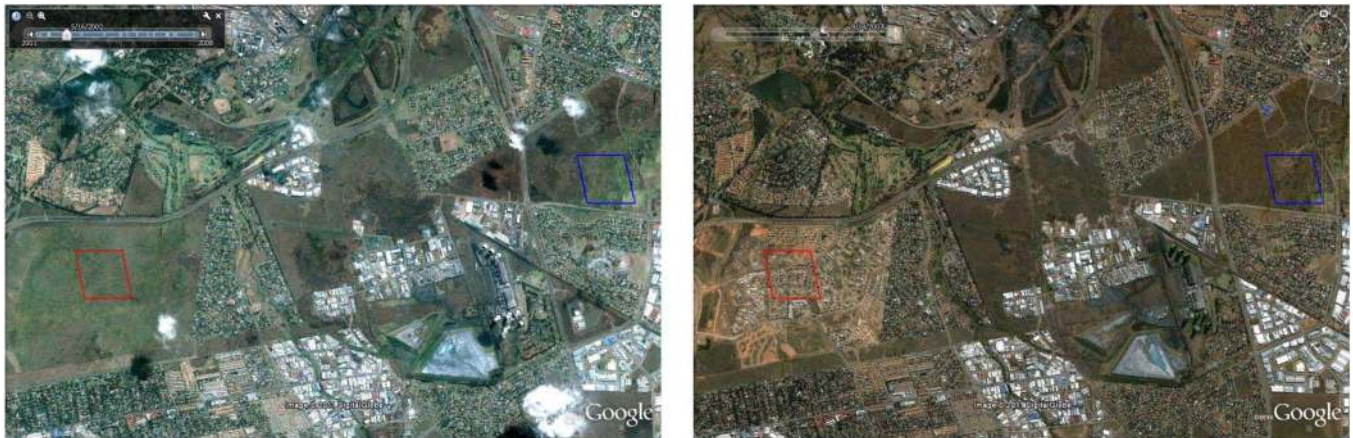
Fig. 1. QuickBird image taken in 2002 (left image) and 2007 (right image) respectively. The polygon on the left in both images is the outline of a 500 m MODIS pixel in an area that changed from natural vegetation to settlement while the polygon on the right in both images is the outline of a 500 m MODIS pixel in an area that remained naturally vegetated. (courtesy of Google™ Earth).
