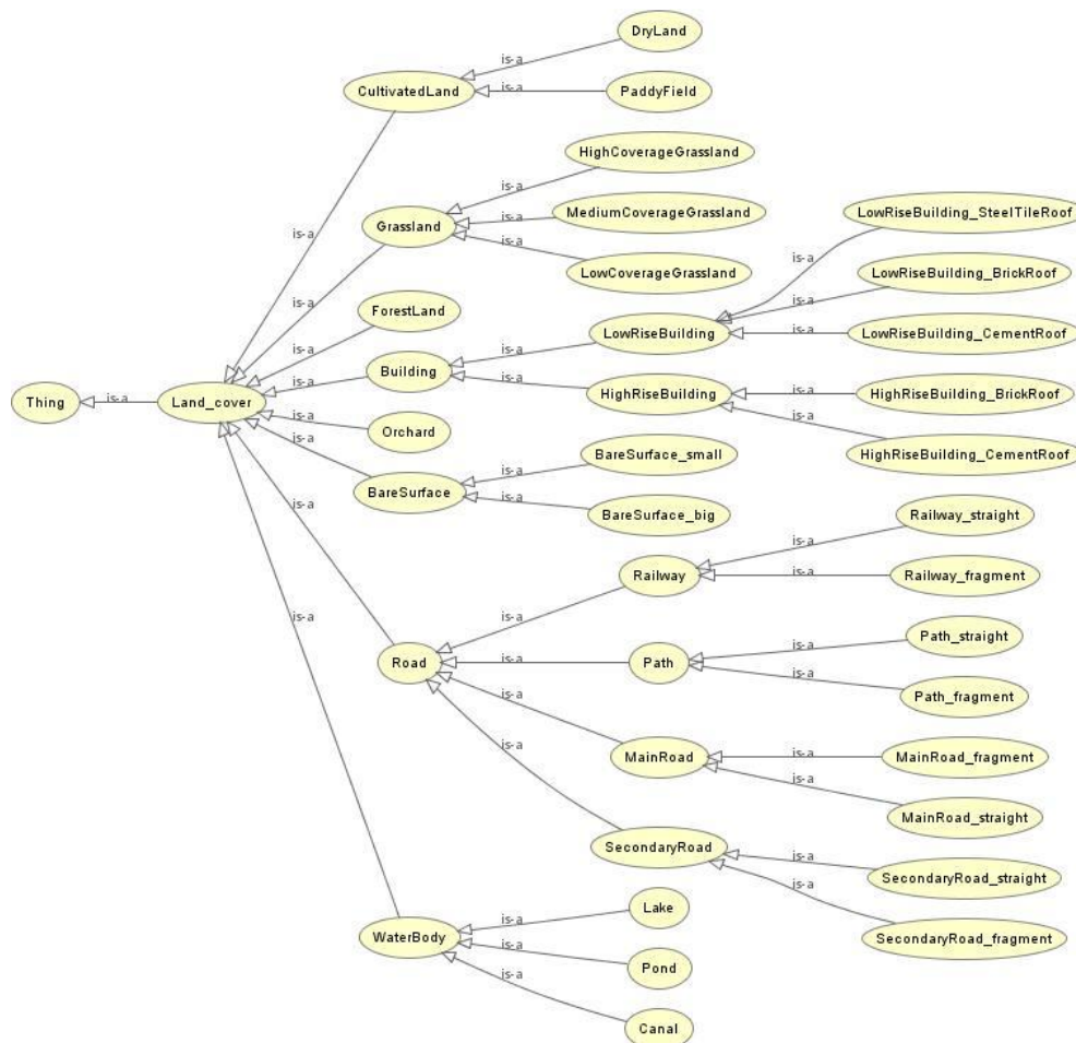
Figure 1. Hierarchy of land cover ontology. According to the China Fundamental Geographic Information Category, land cover classes are selected for the land cover ontology. Land cover classes have the relationship of “is-a” in the ontology hierarchy.
