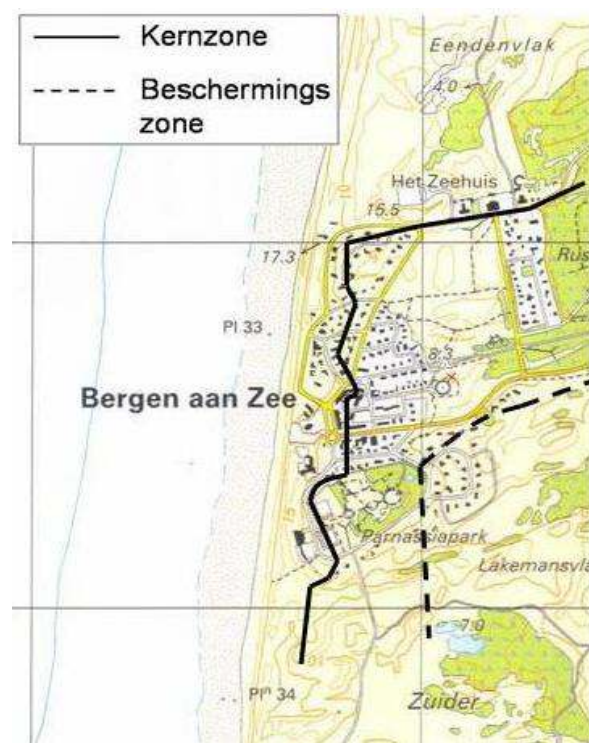
Figure 6.2: Flood defence line (Kernzone) that divides a city into the legally protected and unprotected zone
