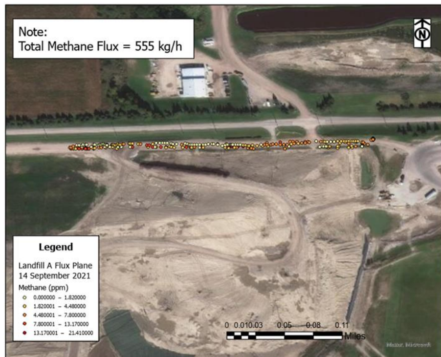
Figure 9. Methane concentrations measured at the downwind edge of Facility A on 14 September 2021, 9:04 a.m. to 9:23 a.m. The height of the flux plane was 35 m.
