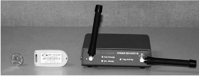
Figure 2. The RFID reader and tag used in our prototype system.
