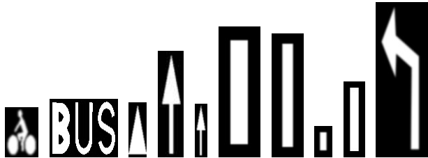
Fig. 3. Library of road marking template patterns ( GSD = 2cm ).
