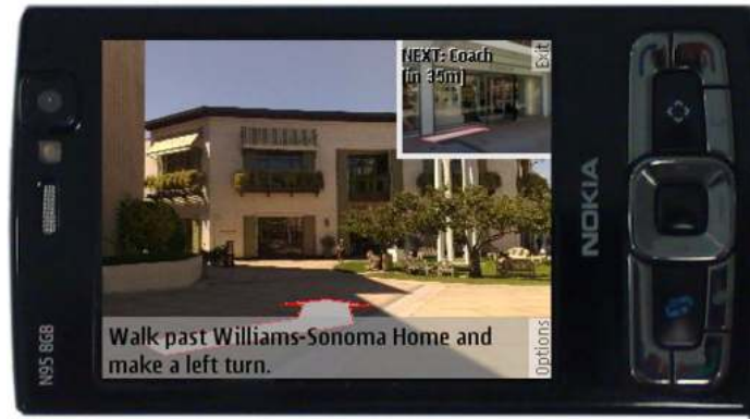
Fig. 2. A sample client view of a generated instruction. The current direction is displayed prominently, but a preview of the next step is shown in the top right corner.
