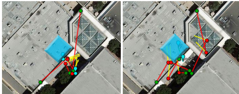
Fig. 10. Left image shows what happens if we apply the original algorithm to the landmark in the left image of Fig. 9. Large GPS error leads to bad pose estimation. Right image shows what happens if we do not perform outlier detection. We get proper orientation but scale is not estimated correctly. This demonstrates the need for our alternative alignment method.
