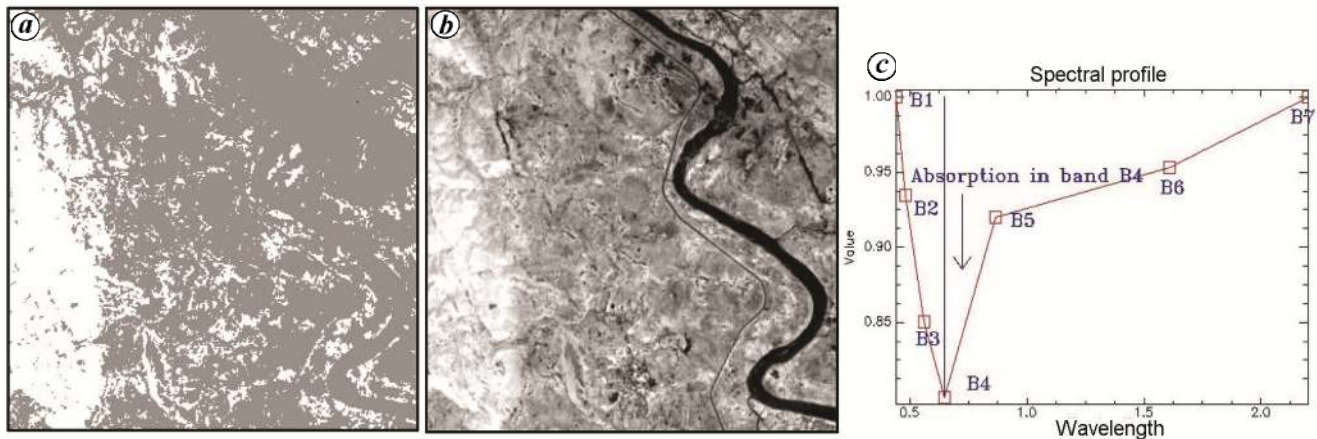
Figure 7. a , RBD image (b2 + b5)/b4 in integer value. b , RBD image (b2 + b5)/b4 in float value. c , Spectral plot showing absorption band.
