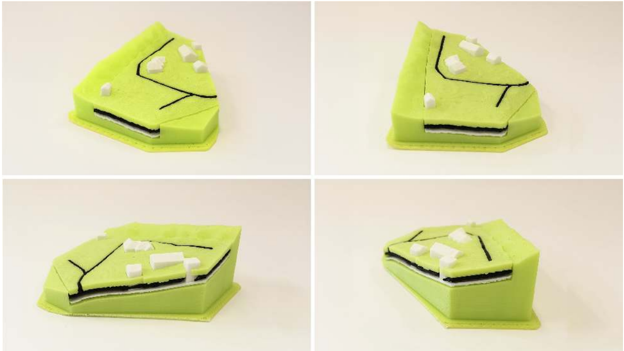
Figure 7.4: Using more indentation, our system can account for accumulated imprecision of stencil layers.
