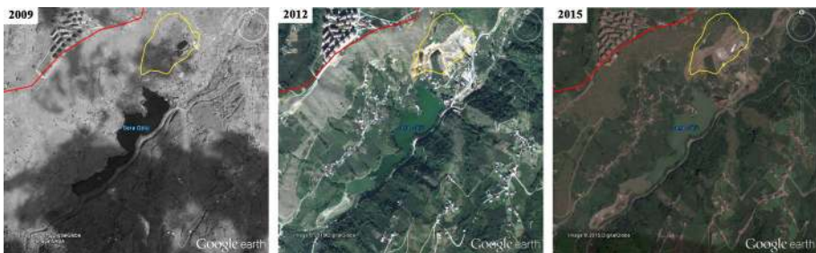
Fig. 3 Aerial view of Lake Sera. Areas north and south of the Basin have seen considerable development leading to deforestation of the forest around thus increase landslide risks. The red line designates the extent of the Sera River Basin and yellow the presently active landslide zone Source: Images obtained from Google Earth
