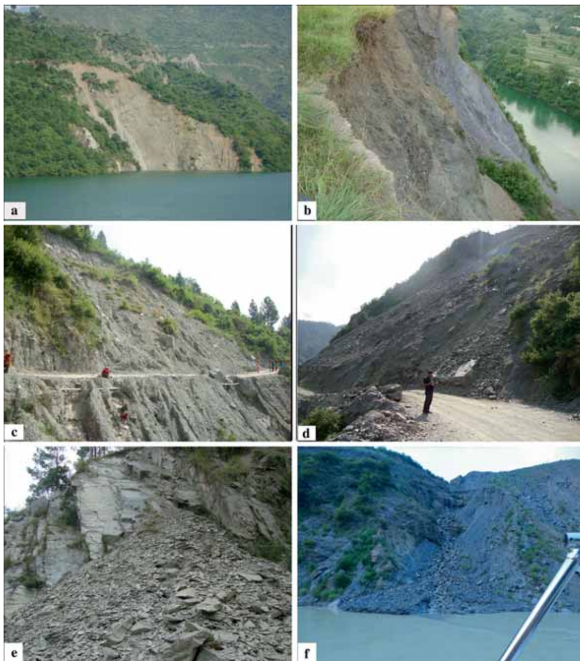
Figure 3. Field photographs: (a) typical arcuate shape scar of the reservoir-induced landslide, (b) slope failure in RBM, (c) rotational failure along the road network, (d) rotational failure in debris along the road and (e) slope form of phyllite is subjected to plain failure and (f) drainage-induced landslide.
